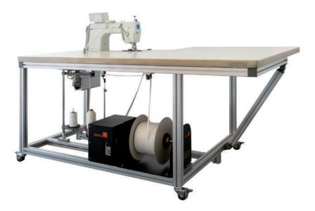
The SM Optima +SEAS is a SEG Keder semi-automatic sewing system that is composed by a high-end lockstitch sewing machine, an optimized sewing table and a SEAS Universal Kit.
