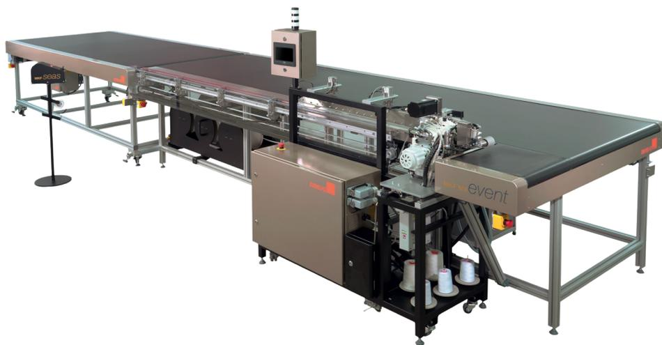
To help handle and align heavy and oversized display textiles, we created the Extension Table. It is possible to incorporate one or two Extension Tables to the MX Event +SEAS, allowing users to have a length of 6 to 10 meters.
