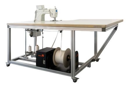
The SM Optima +SEAS is a highly productive semi-automatic sewing machine composed by a high-end lockstitch sewing machine, a SEAS Universal Kit and an optimized sewing table for easy handling of large textiles.
